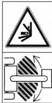
19. Stand clear from the area of the joint hitches when the engine is on.
