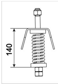
**FIG. 23. TENSIONING OF THE DRIVE CHAIN SPRING LABEL.**
