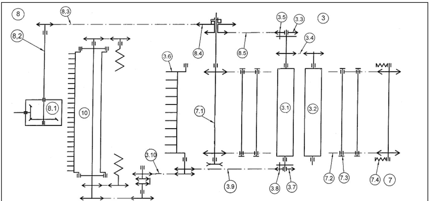
**FIG. 37. DIAGRAM OF THE ROUND BALER DRIVES WITH CHAIN BALING CHAMBER**
