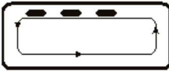
Net wrapping is shown as three elements of the display moving counter clockwise around the edge, as shown in the picture. After cutting the net, the display will show the **Stop** sign again.
