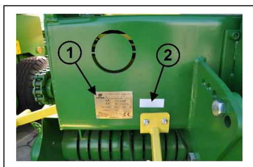
**FIG. 34. VIEW OF THE NAMEPLATE AND THE SERIAL NUMBER OF THE BALER.**
