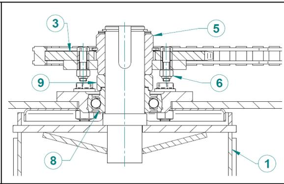
**FIG. 68. SAFETY MECHANISMS OF THE FORK FEEDER AND THE PICKUP, LEFT SIDE OF THE BALER**
