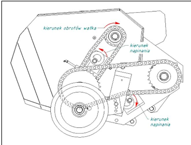
**FIG. 53. ADJUSTMENT OF THE PICKUP DRIVE AND SCREW FEEDER CHAIN (LEFT SIDE)**
