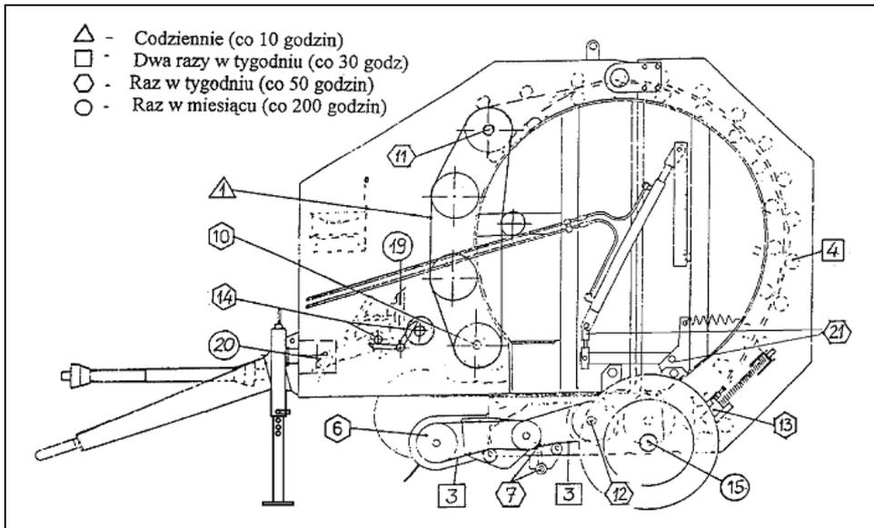
FIG. 73. GREASING POINTS (LEFT SIDE)
