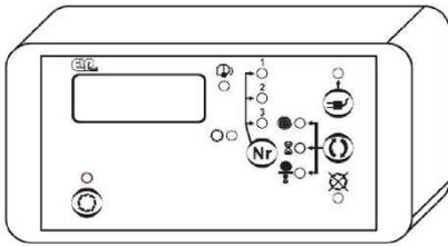
Balers SIPMA PS 1510 FARMA and SIPMA PS 1210 CLASSIC; SIPMA PS 1211 FARMA PLUS may be equipped with a universal controller used for controlling the key operating parameters of the Baler.
