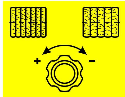
**FIG. 18. LABEL - ADJUSTMENT OF TWINE BALE
