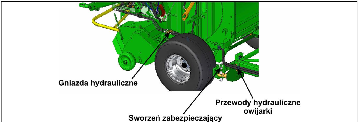
**FIG. 81. COUPLING THE BALER WITH A WRAPPING MACHINE**
