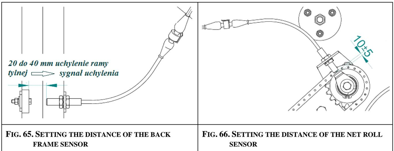
**FIG. 65. SETTING THE DISTANCE OF THE BACK FRAME SENSOR**
