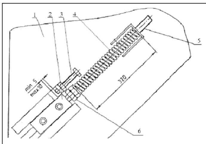
**FIG. 50. ADJUSTMENT OF THE BALING CHAINS**
