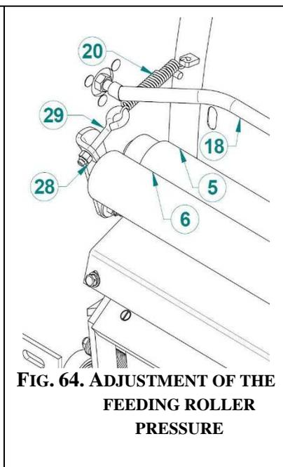
**FIG. 64. ADJUSTMENT OF THE FEEDING ROLLER PRESSURE**
