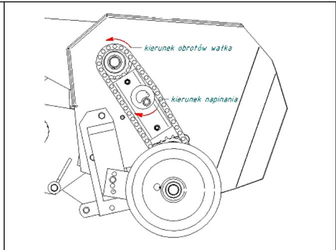
**FIG. 54. ADJUSTMENT OF THE SCREW FEEDER DRIVE CHAIN (RIGHT SIDE)**
