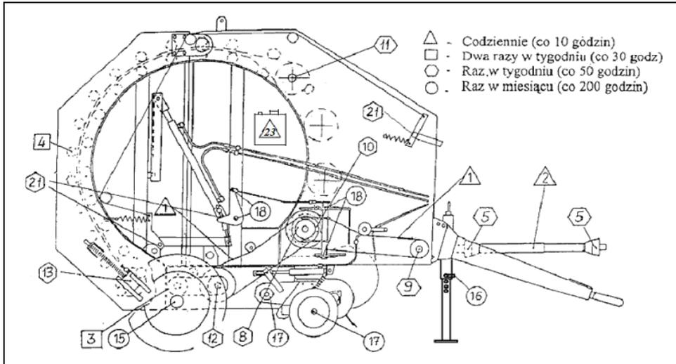
FIG. 72. GREASING POINTS (RIGHT SIDE)
