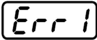
Short circuit on the reed sensor power supply. The device must be immediately switched off with any key and the fault must be removed.
