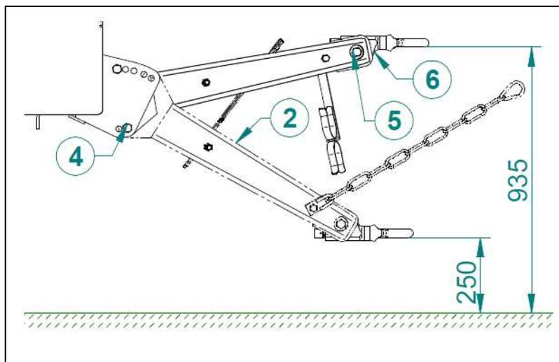
**FIG. 44 ATTACHING THE BALER TO THE UPPER TRANSPORT HITCH**
