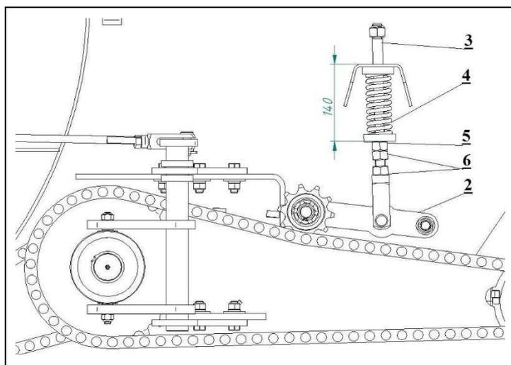
**FIG. 51. ADJUSTMENT OF THE MAIN DRIVE CHAIN**
