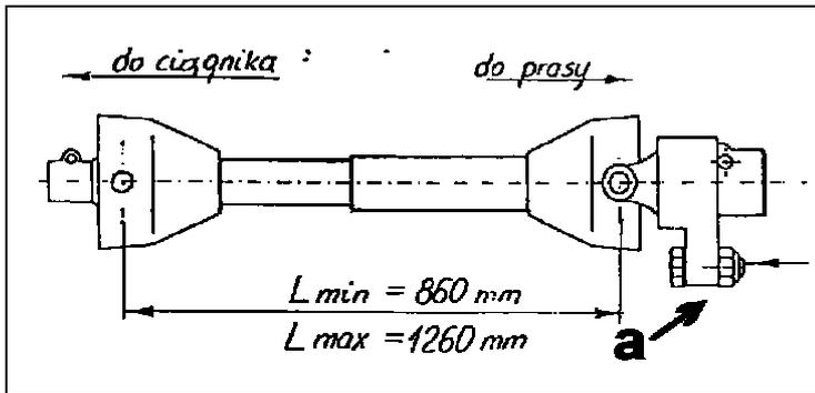
**FIG. 45. ARTICULATED TELESCOPIC SHAFT WITH FLANGE COUPLING**
