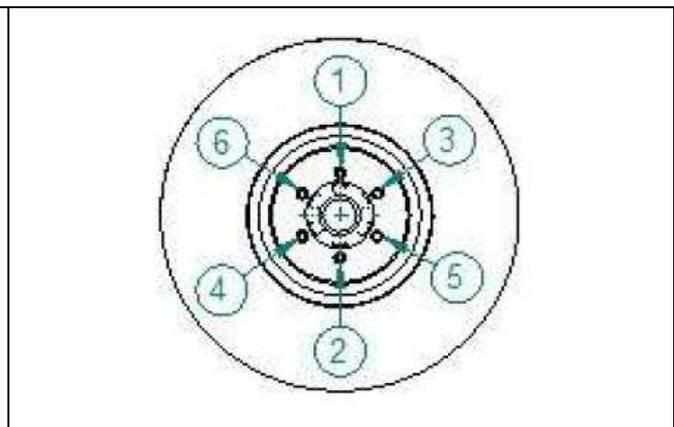
**FIG. 76. POINTS WHERE A LIFT IS POSITIONED WHILE DISASSEMBLING THE WHEELS**
