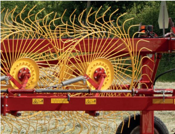
The standard version has rake wheels with a diameter of 55" (1.4m) and tines with a diameter of 0.28" (7mm). As an alternative, and with no changes to the machine structure needed, it is possible to mount optional rake wheels with a diameter of 60" (1.52m) and tines with a diameter of 0.3" (7.5 mm). Each wheel, regardless of the diameter, is equipped with 40 tines made of top-quality spring steel.
