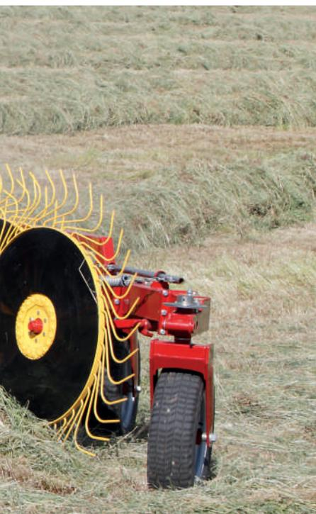
In order to adapt to extreme field conditions, hay rakes must be solid and sturdy. This is why the drawbar and the rake wings have been made using a large lattice framework of structural tubing to make them tough and fully reliable over time, however hard they are made to work. Despite their size, these machines are easy to handle and transport and very user-friendly.
