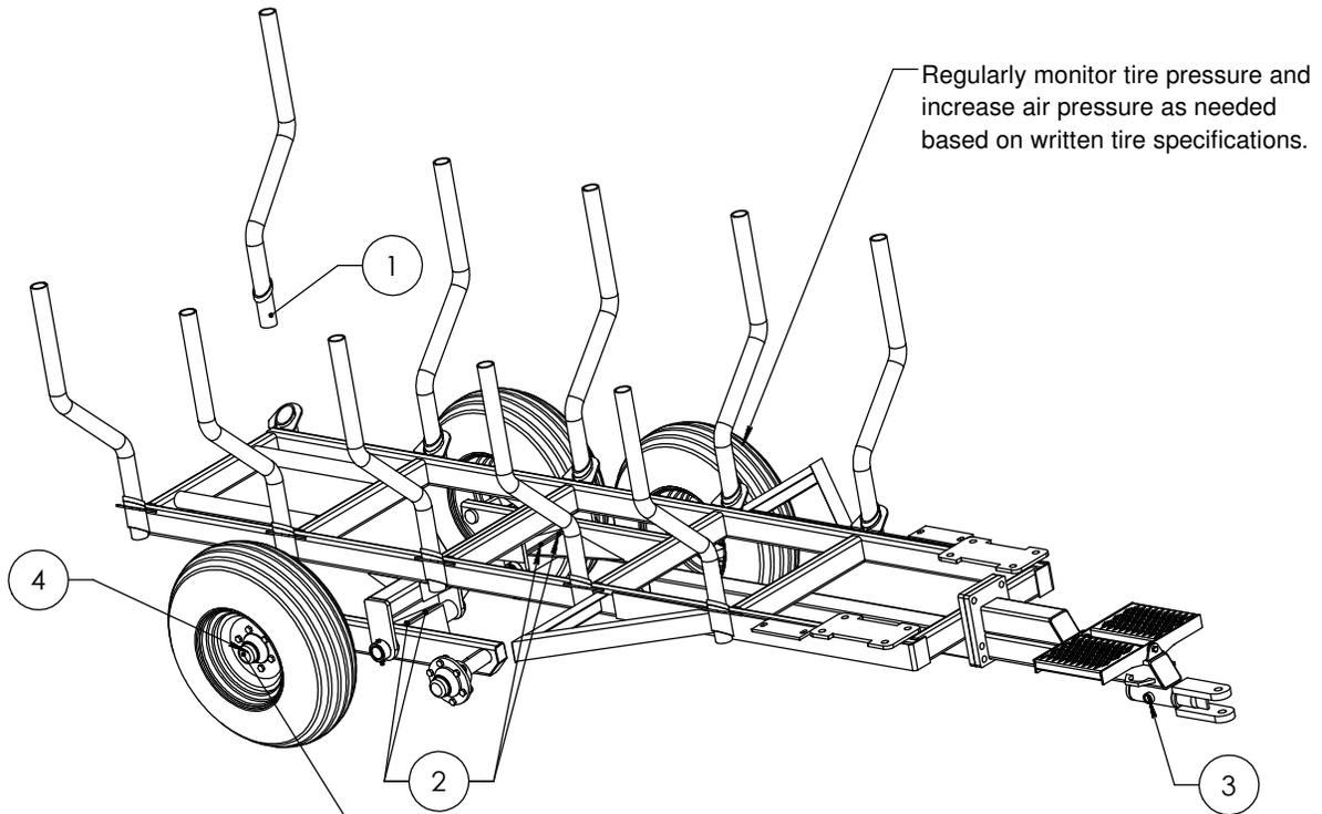
By prevention, remove the cap once a year, tighten the castellated nut, fill the cap with grease and replace the cap!
