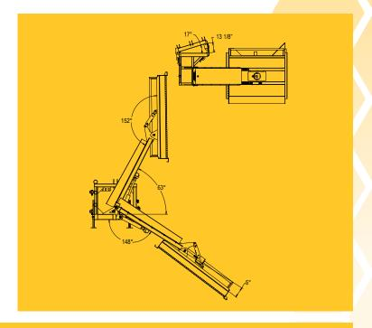
Woody's lateral or side brushcutters are specially designed for maintaining the edges of agricultural fields and forest paths. Mounted on a 3-point hitch, they feature a front and transverse frame made of Hss 50W 1/4. The cutter itself is constructed with 3/16 and 1/4 inch 50W plate. With its robust design, it can effectively cut branches up to 3 inches in diameter, providing a versatile solution for managing bushes, shrubs, and small trees across large areas.
