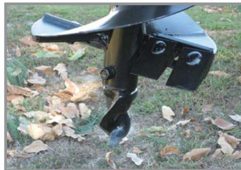
**Augers** — Fishtail center point and high carbon, alloy steel digger teeth offer dependable operation with long component life. Augers range in diameter from 6" to 30" single or double flight, standard duty or heavy duty with reinforced collars and heavier flighting allows the operator to choose the auger that is right for the job.
