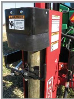
**Rubber Shield** — First to install rubber shield around ram driving head, reduces flying wood chips and debris.
