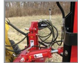
**Hydraulic Adjustable Mount** — Hydraulic Adjustable mount with 3" x 6" cylinders provides superior ram control with trouble-free performance.
