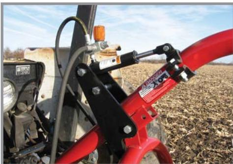
**Optional Down Force Kits** — Provide 350-500 lbs. of extra pressure, increasing performance in tough digging conditions. Available for models 500, 720 and 925 post hole diggers. (not for small, compact tractors)
