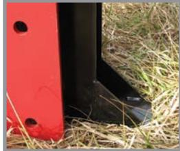
**BigFoot Stabilizer Leg** — Standard on HPD-16/22Q/26Q SHC, Big-foot stabilizer provides sure footing for driving those larger posts, reducing the driving shock load to the tractor.
