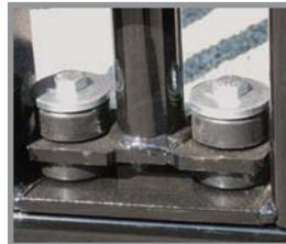
**Cushion Mount** — Cushion mounts on Q-series drivers reduce spring vibration and driving ram shock resulting in increased reliability.
