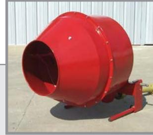
Worksaver's Skid Steer Mixer, model SS-590 has direct hydraulic drive of the gearbox which eliminates chain and sprocket maintenance resulting in more up-time on the jobsite. Large 11-cubic ft. drum allows the operator to mix, transport and place 5-cubic ft. of concrete. It's efficient design offers the contractor a cost savings over chain driven models.
