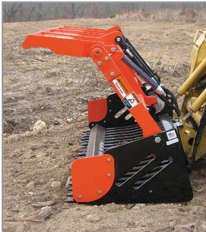
(Right) Bolt-on side plates hold smaller rocks in the bucket. They can be removed from the bucket to allow the SARG to handle logs and stumps.
